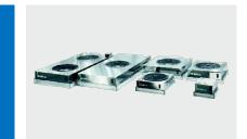
Fan Filter unit (FFU) is a leading edge FFU unit designed to provide filtered laminar air flow over a specific area. The unit integrates a high efficiency fan together with a HEPA filter. The FFU draws in contaminated air from top of the module and exhausts filtered clean air vertically class 100 to class 100000 clean rooms. ISO-Class 5 (as per ISO Standard 14644-1)
