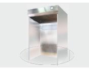
Reverse Laminar Air Flow is used to control the hazardous emissions of powder dust during powder dispensing/sampling processes without any risk to operator and products as well protecting the environment. The down draught of HEPA filtered air prevents airborne dust caused by handling operation away from the operator breathing zone. Three levels of air filtration is carried out into the booth air stream.
