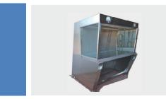
Horizontal Laminar Air Flow is localized clean air station to carry out various test under ISO Class 5 (ISO std. 14644-1) filtered air. Horizontal Laminar Air Flow is used when non toxic and nonflammable tests are carried out. Laminar Unit also consist of UV light, UV hour meter, Steripot as per requirement. Sometimes antistatic grill is provided to remove the static charge as per process requirement.
