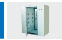
Air showers are used at entrance of dust free premises. High velocity clean air bath is created inside air shower chamber to remove dust particles from human body ,clothes and material if carried out through the air shower. It is a barrier by door interlocking between internal & external environment to avoid the dust. It is used as recovery unit also in gold industry. Gold dust trapped in HEPA filter is recovered by burning the HEPA filter.
