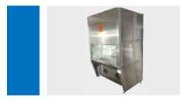
Bio-safety cabinet is used to protect product, personnel and environment. Mostly it is used when risky microorganisms are handled. Most widely used Bio-Safety Cabinet are of class-II type A and B. Class-II A type Bio-Safety cabinet have partial exhaust i.e. 30% and 70% recirculation and class IIB type Biosafety cabinet have 100% exhaust. Class II B Biosafety cabinet is used when most toxic or radioactive substance are handled.
